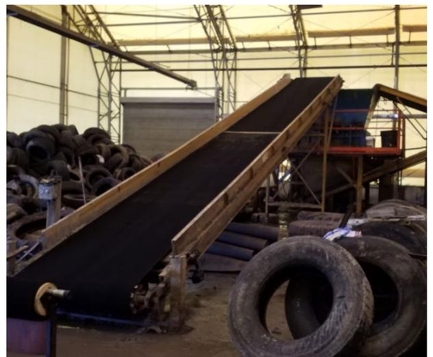
Freshly installed conveyor belt on Bolder Industries SSI primary shredder system
